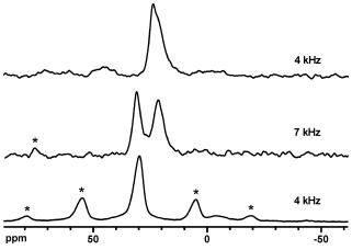
Figure 3. <sup>31</sup>P CP/MAS NMR spectra of [1a(II)Et<sub>2</sub>]<sup>2+</sup>·2BF<sub>4</sub><sup>-</sup> (top trace), 1a(II)(AuCl)<sub>2</sub> (middle), and 1a(AuCl)<sub>4</sub> (bottom). \*rotational sidebands.
