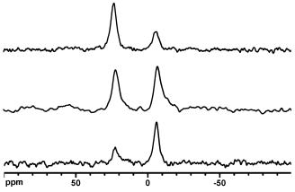
Figure 1. <sup>31</sup>P CP/MAS NMR spectra of 1a(II) (top trace) and 1a(I) (middle). Bottom trace: <sup>31</sup>P MAS of 1a(I). Rotational frequency 4 kHz.
